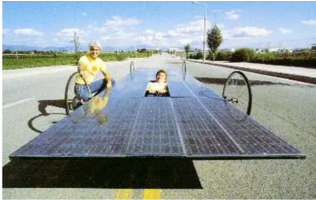
Sunrunner 1.2kW solar arrav (no batteries)
