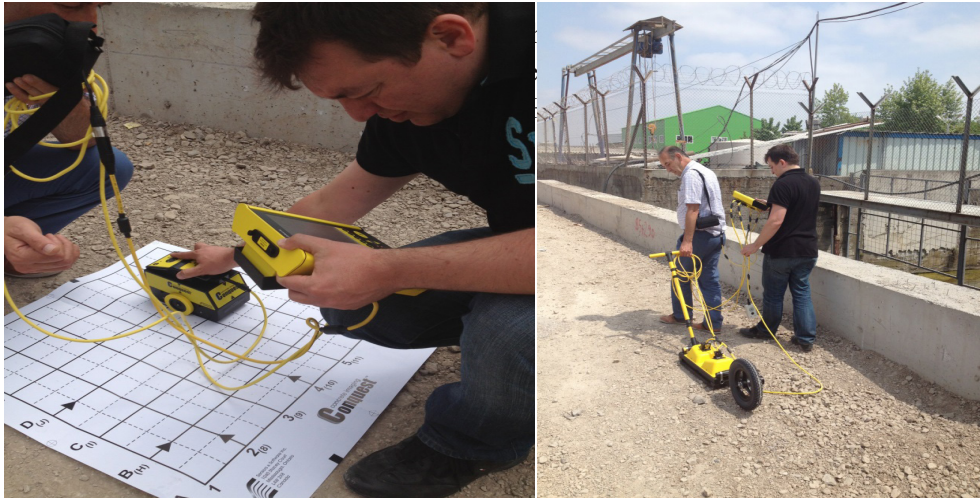
Figure 5. GPR different antennas: with Conquest (2 GHz) Antenna (left); Noggin (500 MHz) Antenna (right) [22]
