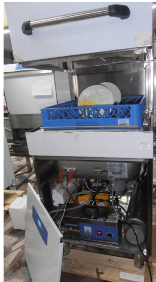
Figure 10. Innovative eco friendly commercial dishwasher system using ozone (front view).
